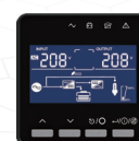
The 3.5 inch touch screen LCD panel can be rotated (Touch screen is gravity sensing)
